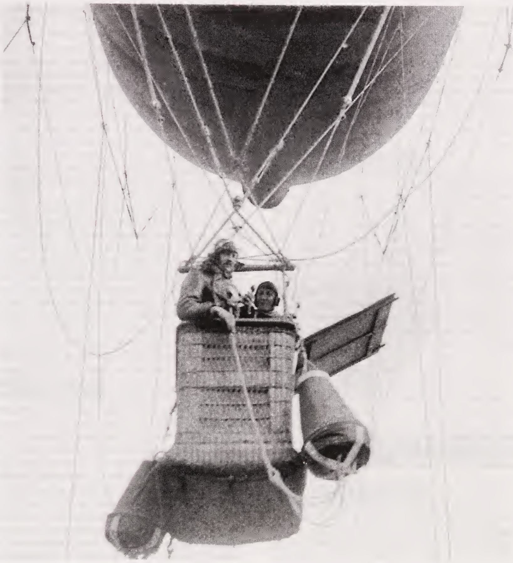
Two observers in a British balloon prepare to search out targets in German-held territory. Note their telephone microphones, large map board, and two parachute canisters—for hasty evacuation if their balloon is attacked by German fighters. (IMPERIAL WAR MUSEUM)
