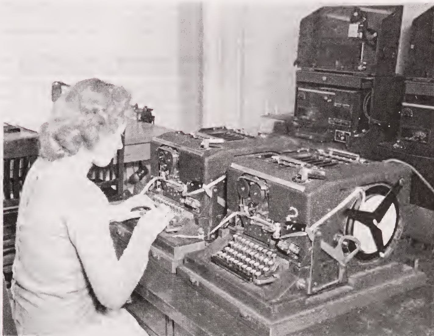
Paired Sigaba machines; the rotor “basket” fits into the top of the machines. (NATIONAL SECURITY AGENCY)
